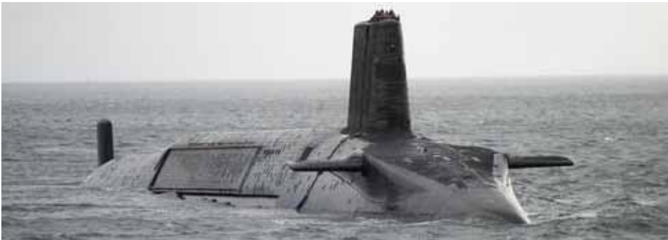
A Royal Navy Vanguard-class submarine on patrol in the Atlantic. It can carry up to 16 Trident missiles, each carrying up to 12 nuclear warheads.
