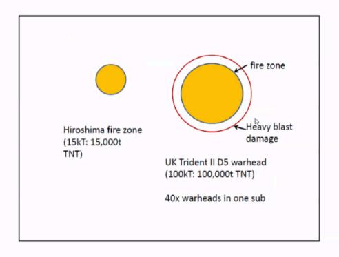
Trident warhead fire zone: approx. 4 times larger in area; scales to the power of 0.8. Blast zone scales to the power of 2/3 (volume effect).
