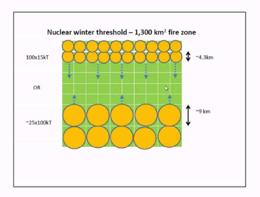
Schematic of 100 Hiroshima fire zone area - equivalent to  $^{\sim}25$  Trident D5 warheads. Postol suggests a possibly 4x larger Trident fire zone than using thermal intensity scaling – scaling to Hiroshima compensates for this.
