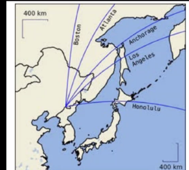
Figure 4 Map showing North Korea and adjacent countries and the initial ground tracks of ICBMs launched from north-central North Korea to five cities in the United States. ICBM ground tracks differ from great circles connecting the launch site to the target because of Earth's rotation. Cf. [APS 2003, Fig. 5.8].
